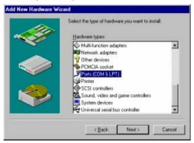
10 Documentation No.3PXCC1x-2x-3903 B&B Electronics Mfg Co – 707 Dayton Rd - PO Box 1040 - Ottawa IL 61350 - Ph 815-433-5100 - Fax 815-433-5104 B&B Electronics Ltd – Westlink Comm. Pk – Oranmore, Galway, Ireland – Ph +353 91-792444 – Fax +353 91-792445 Select (Standard port types) and Communication Port. Click Next.
